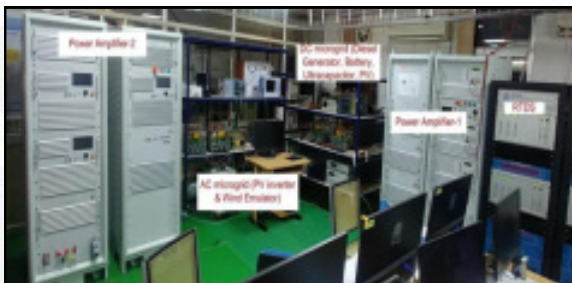
Figure 70: AC-DC Hybrid Microgrid Laboratory test bed
